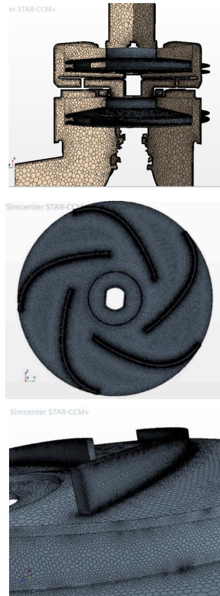
FIGURE 5: MESH STRUCTURE OF THE SUBJECT PUMP
