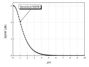
**Fig. 2** SQNR<sup>s</sup> dependence on  $\mu/\sigma$  for symmetrical quantizer design
