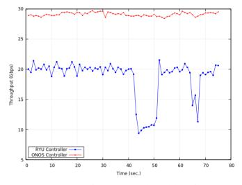
Fig. 3 TCP throughput between the farthest hosts (h1 and h32) for the proposed topology with RYU or ONOS controller
