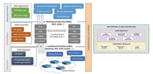
Fig. 1 Overview of a typical layered SDN architecture (left) and SDN controller architecture (right) [3]
