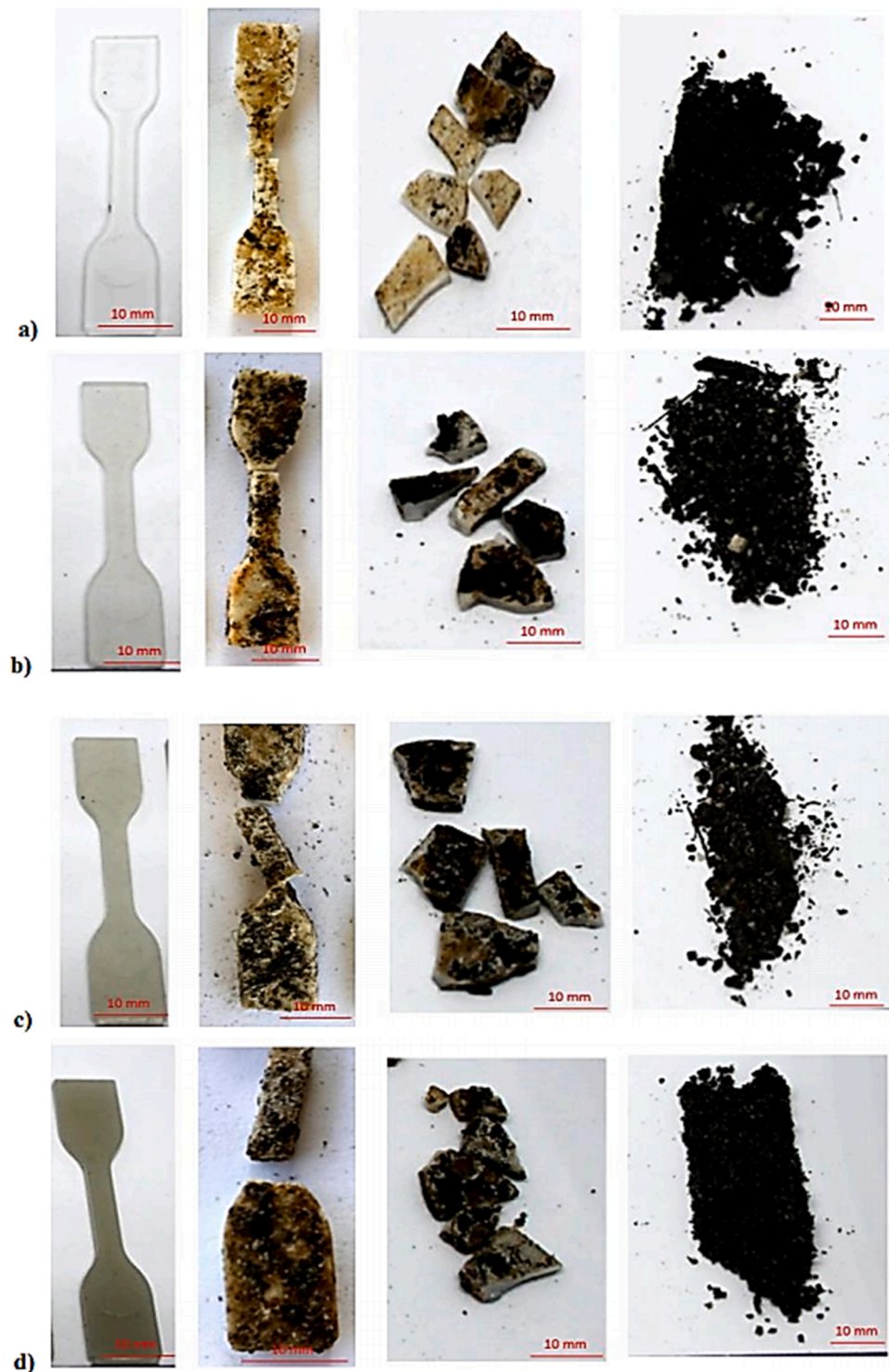
Fig. 11. Macroscopic view of biocomposites before and after 30, 60, and 90 days of composting using the C2 technology. PLA (a); PLA/1HNT/C2 (b); PLA/2.5 HNT/C2 (c); PLA/5HNT/C2 (d).
