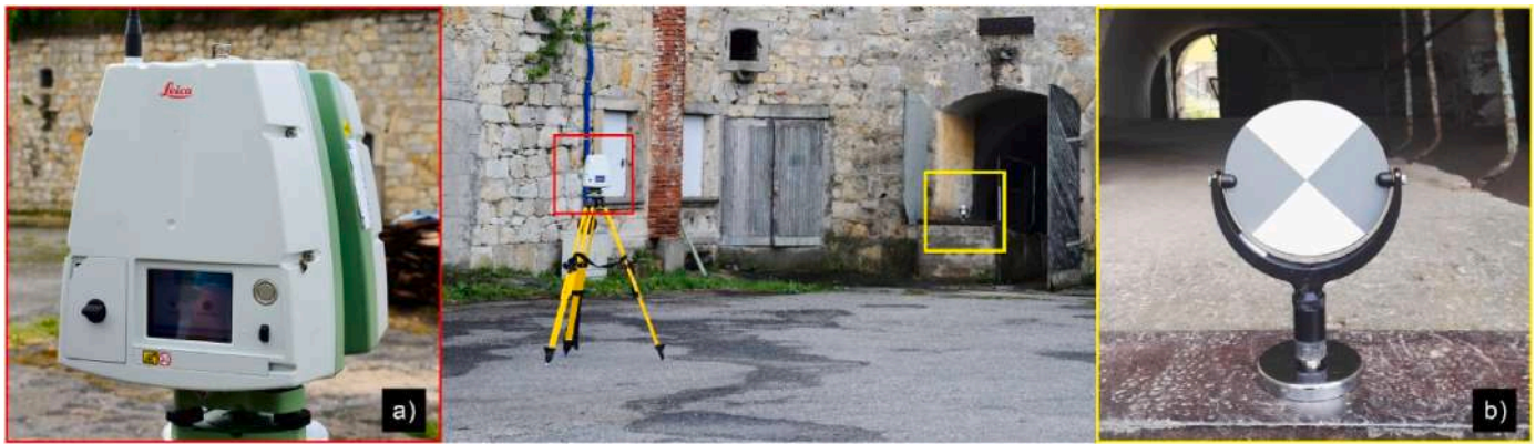
Fig. 7. Alignment of the measuring device (a) and the target plate (b) during measurements - authors' elaboration.
