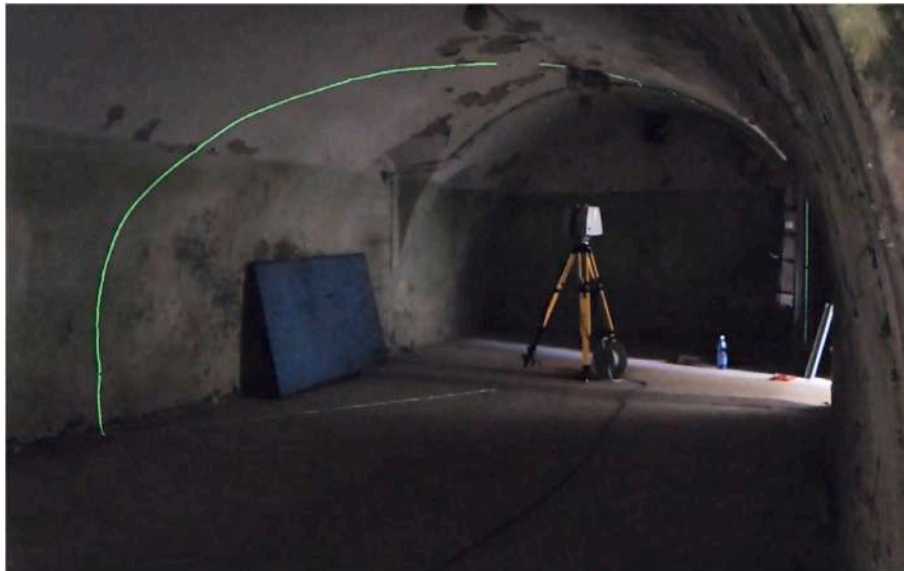
Fig. 3. Leica ScanStation C10 during measurement with a laser beam – the authors' photography.
