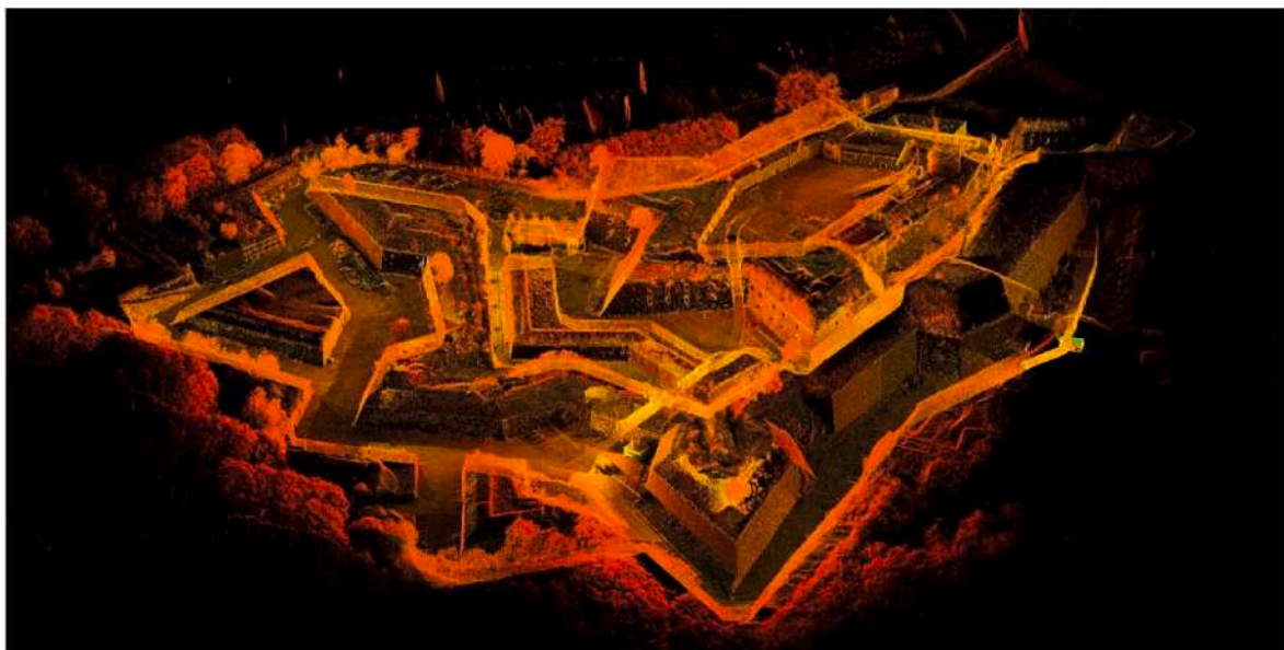
Fig. 10. Point cloud representation of Klodzko Fortress generated with Leica Cyclone software - the authors' elaboration.
