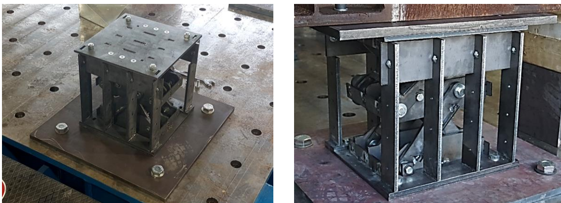
Fig. 2 – Kinematic Steel Joint (KSJ) isolator prototype.
