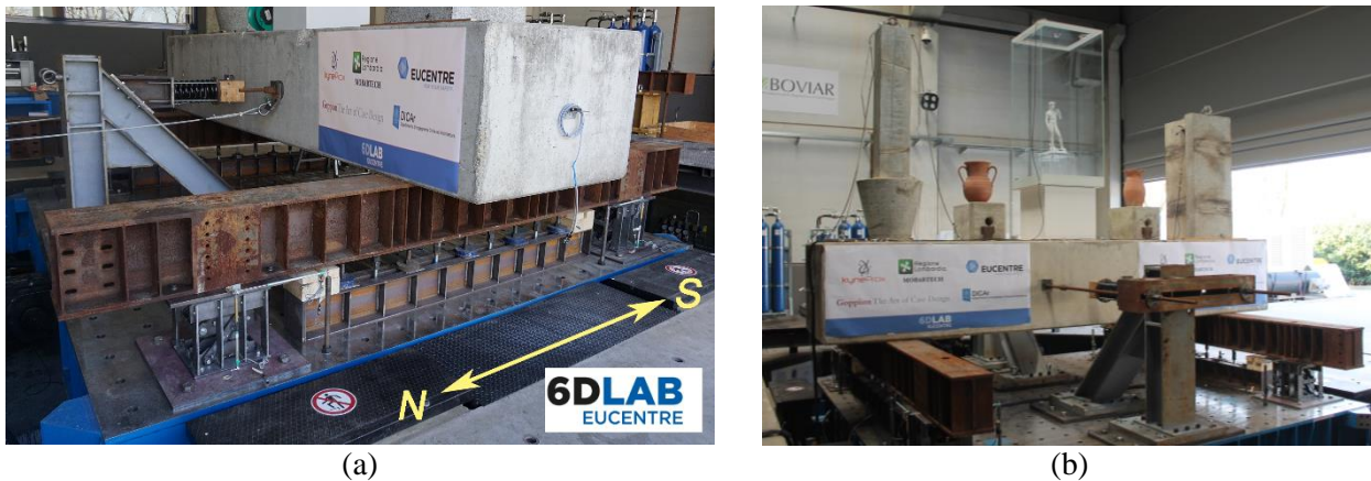
Fig. 4 – Shake-table test setup: (a) isolated configuration; (b) fixed-base configuration.
