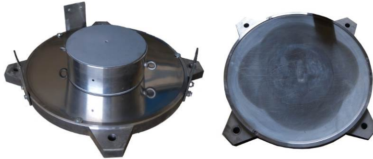
Fig. 2 – Double Concave Surface Slider (DCSS) device: realized device
