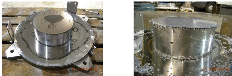
Fig. 13 – Wear evidence – DCSS-D260 material A (left) and material B (right)
