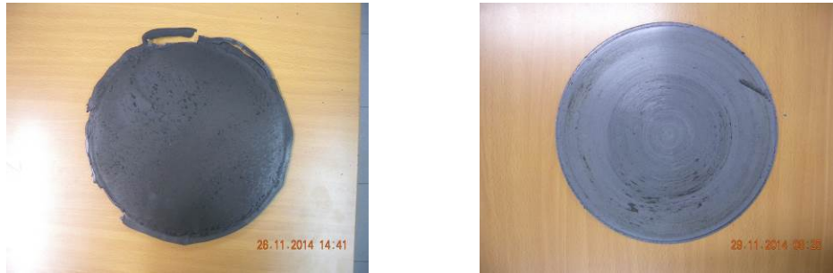
Fig. 12 – Wear evidence – FS-D260 material A (left) and material B (right)
