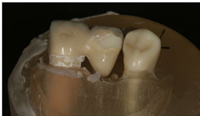
Fig. 6 Failure after TCML (example group III)
