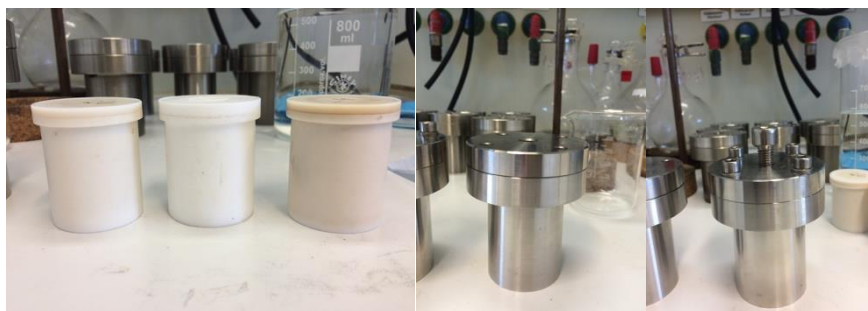
Figure 1.7. (a) Teflon containers used in the synthesis of MOFs. (b) Stainless steel containers (autoclaves) used in the synthesis of MOFs.
