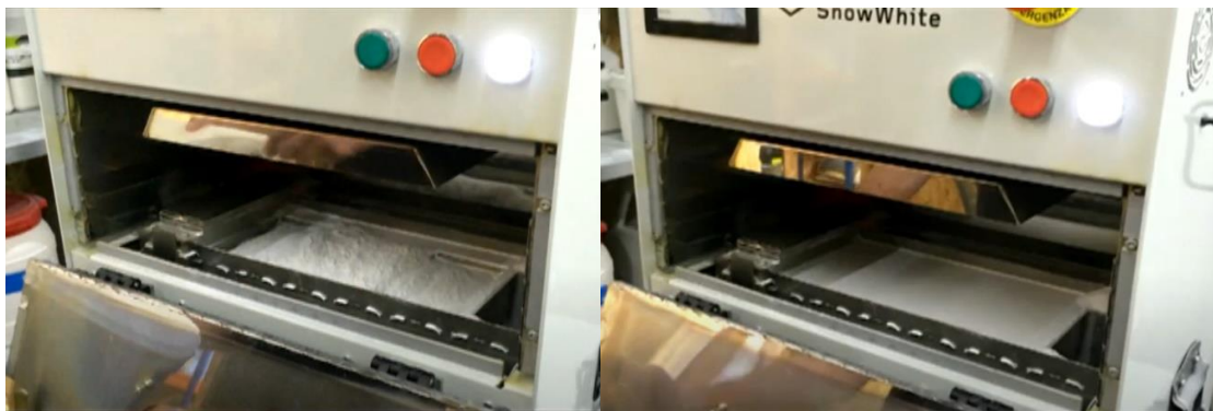
Figure 2.10. The module of sample preparation filled with polymer.
