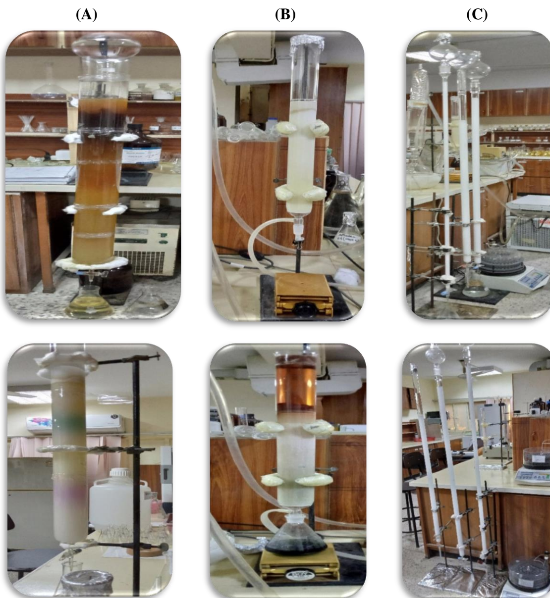
Appendix (5): Column chromatography to obtain purified bioactive compounds as (A) silica gel column, (B) C-18 column and (C) Sephadex column.
