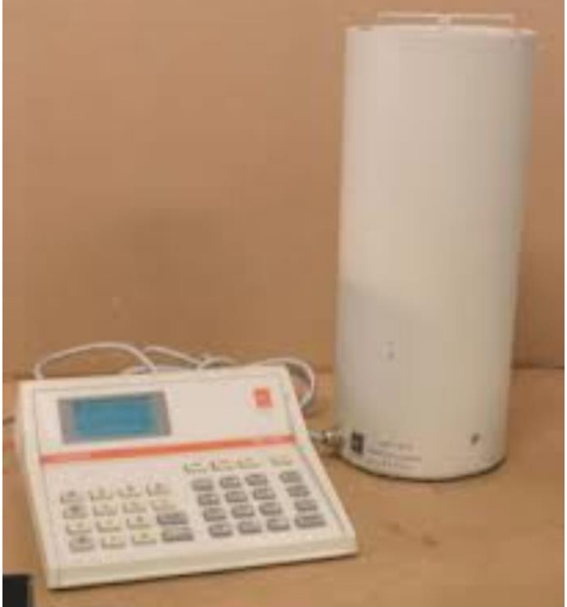
Figure(2.2) Dose Calibrator NMDC(manufacture: BIODEX model:086-336)
