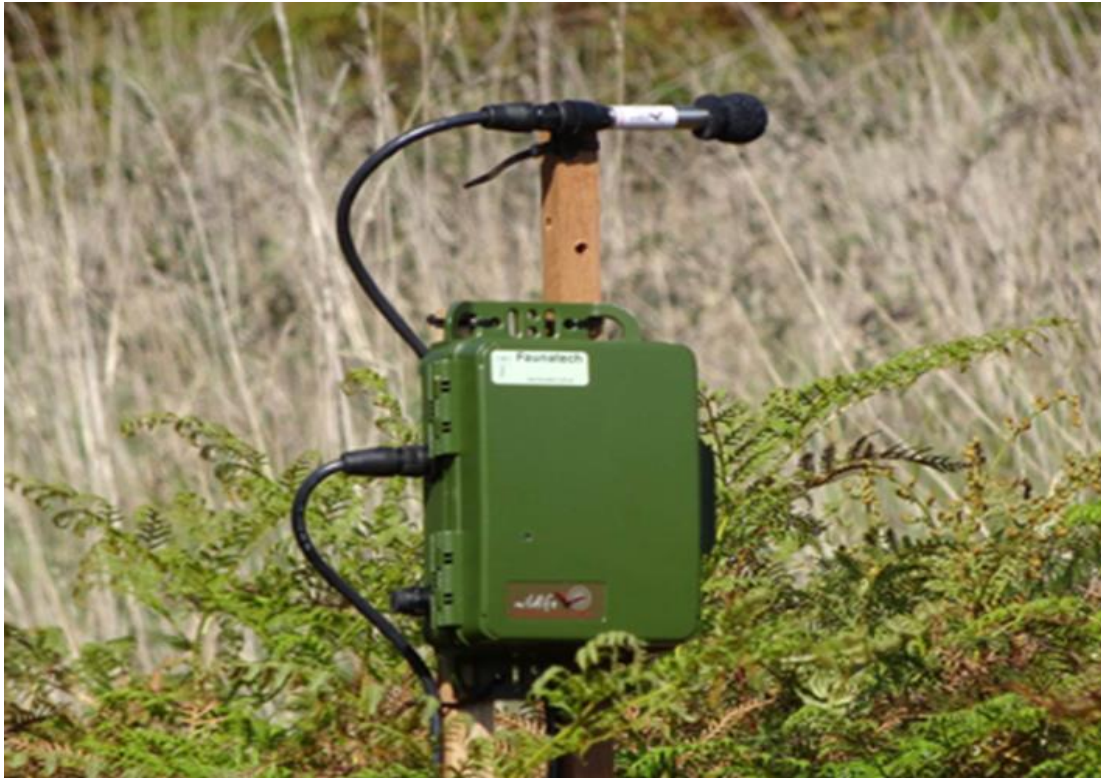
Figure 5- Example of the passive acoustic recorder used for recording audio at the study site.
