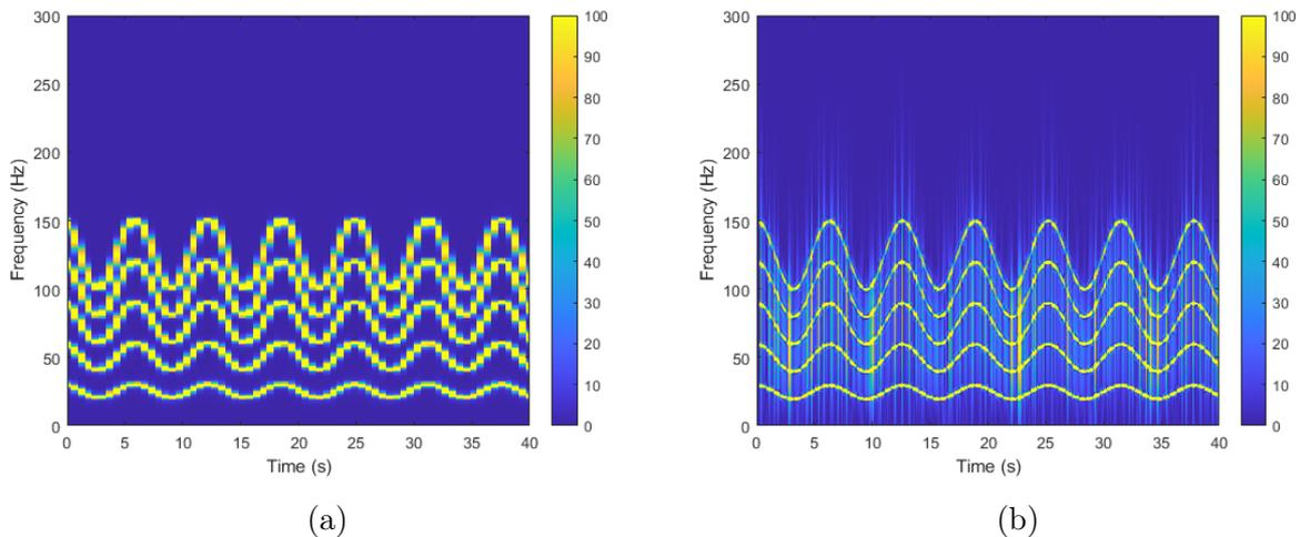
Figure D.2: Numerical example -  $c = 1$  and window 1 s - (a) STFT and (b) CWD
