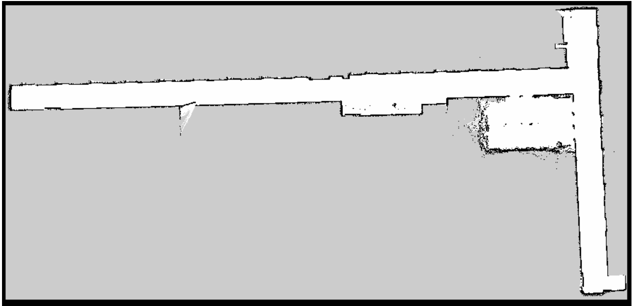
Figure 4.12: Map of the mechatronics department at UiA using Uiabot and SLAM toolbox.
