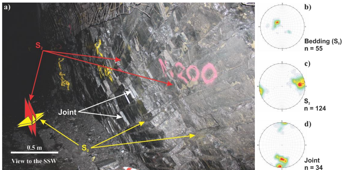
Fig. 2.5: a) Part of a large amplitude F_1 and F_2 Type 1 interference fold preserved in a low strain domain in the North Mine (grid reference 3B). Here, over successive levels, the interaction of three prominent planes results in the development of rhomboid blocks. Photo was taken in the approximate position of the main shear zone. b, c, d) Equal angle, lower hemisphere stereoplots of S_0 (b), S_2 (c) and joint (d) from levels N125 – N220 (125 – 220 m below surface). S_0 has a consistent southeast dip and small-scale low-angle thrusts are developed within the beds and propagate between them. Steep, S_2 undulates with dominant west dips and is marked by thin, sulphide veins, which combined with the chlorite alteration, causes slabbing along the S_2 planes. The joint set has a general north dip and occurs orthogonal to the bedding.
