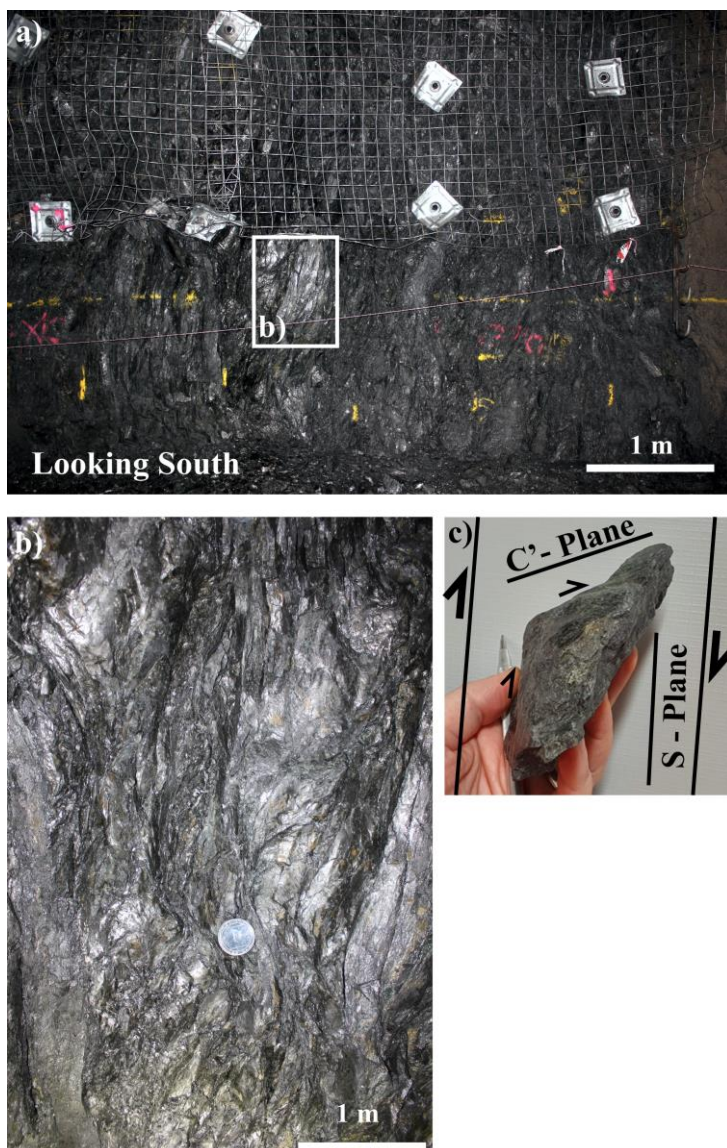
Fig. 3.5: S-C' fabric developed within a D 4 -related high strain zone. a and b) The principal displacement zone on the S390_XC395_W level has a localised steep, east dip (grid reference: 4E). c) Example of a sigmoidal lens created by the interaction of S-foliation and C'-planes.
