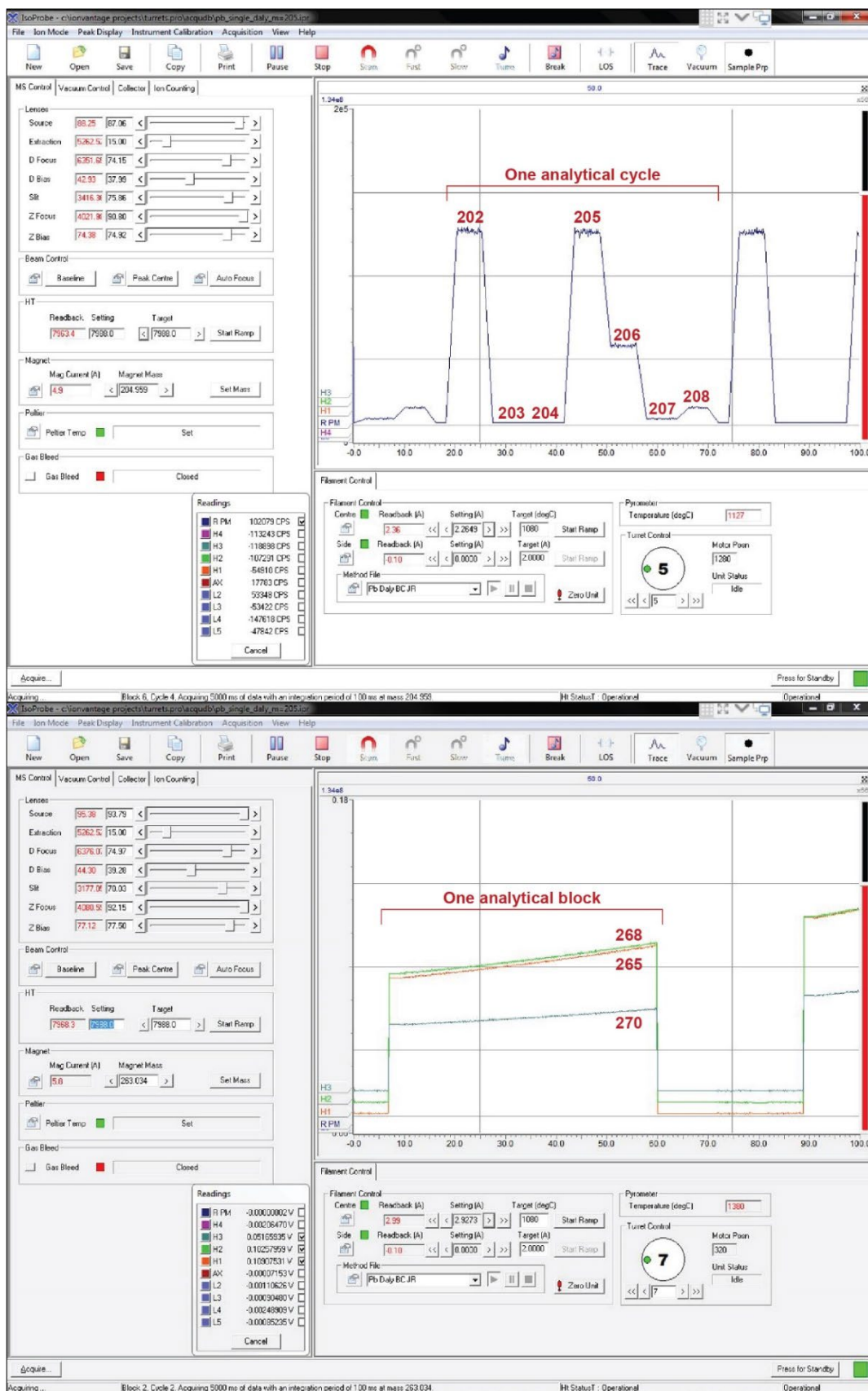
Fig. 2.10 IsoProbe displays during the analysis of lead (top) and uranium (bottom). The measured isotopic masses are annotated in red where Pb isotopes are measured sequentially (separate peaks) with 14-16 cycles per block, and U isotopes are measured simultaneously (as oxides).
