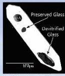
SEM backscatter image of a volcanic zircon with a fresh and a devitrified glass melt inclusion.
