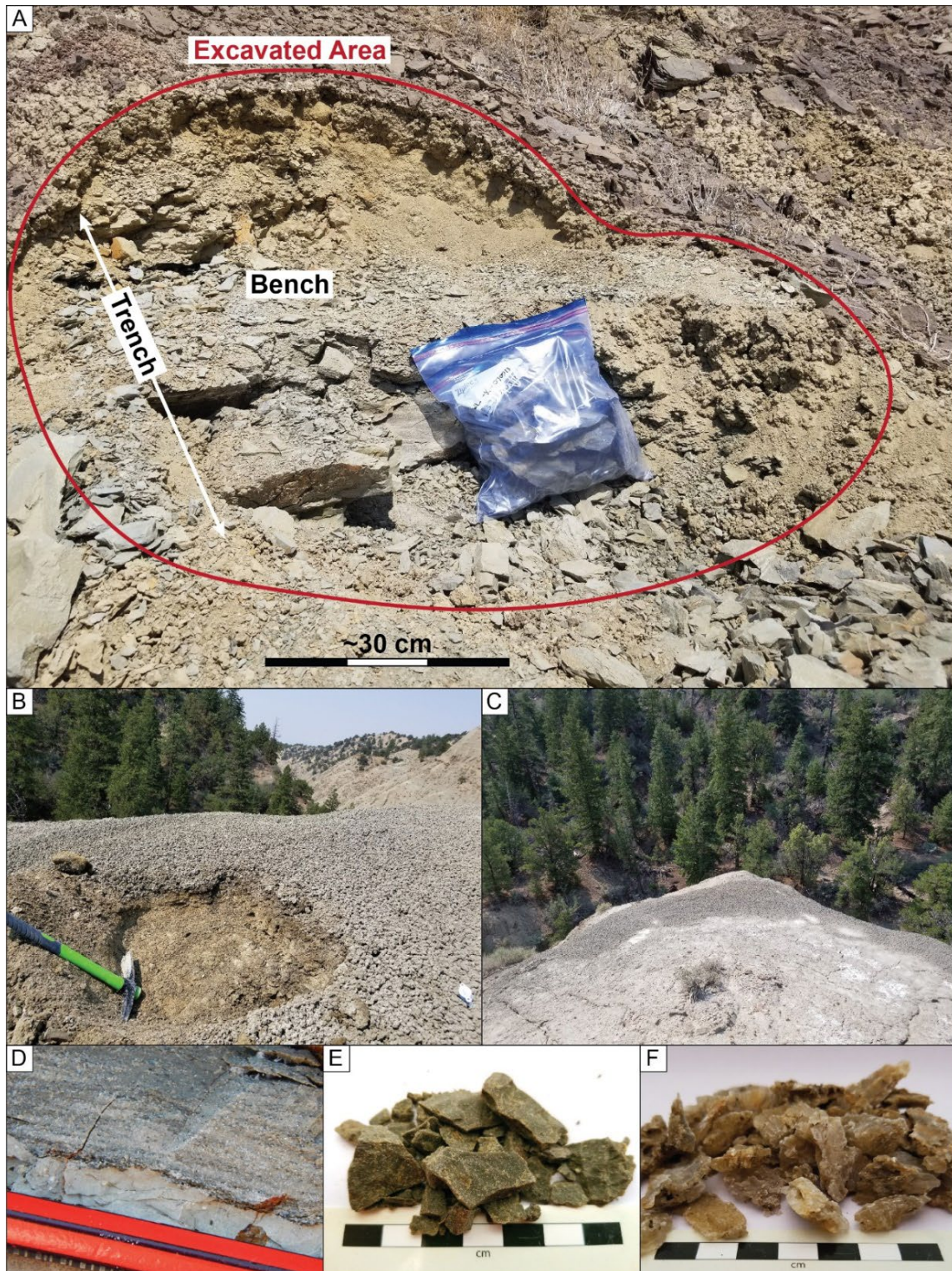
Fig. 2.2 Examples of bentonite outcrops and more. A) Bentonite collection site illustrating the trench and bench approach. B) Bentonite outcrop showing the classic popcorn weathering texture. C) Outcrop in panel B from a distance showing the texture/color change from mudstone to bentonite and the bench-forming nature of bentonite horizons (photograph looks down onto the bench that sits atop a ~20 m cliff). D) Accumulation of phenocrysts at the base of a bentonite horizon deposited in a shallow pond (pencil for scale). E) Bentonite hand sample (smectite chips) illustrating the common pistachio green color and waxy texture. F) Gypsum crystals collected from a bentonite outcrop (slightly rounded during post-collection transport).
