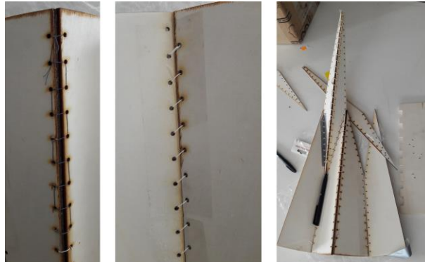
Fig. 20. Plywood stitching (Source: Authors)
