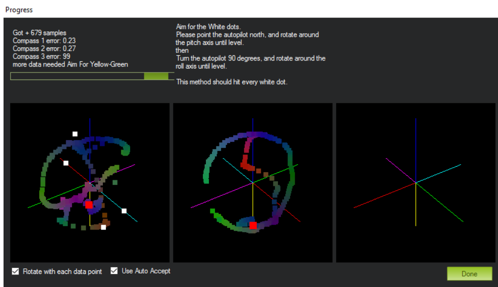
Figure 3.12 – Mission Planner’s compass “Live Calibration” window (Ardupilot Dev Team, n.d.-c).
