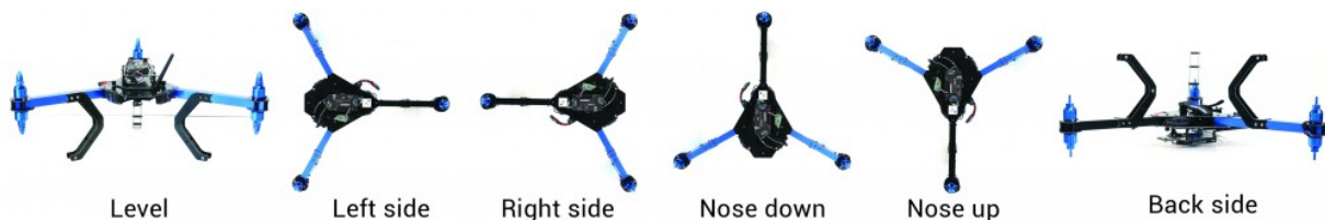
Figure 3.11 – All UAV positions required for successful calibration (ArduPilot Dev Team, n.d.-b).
