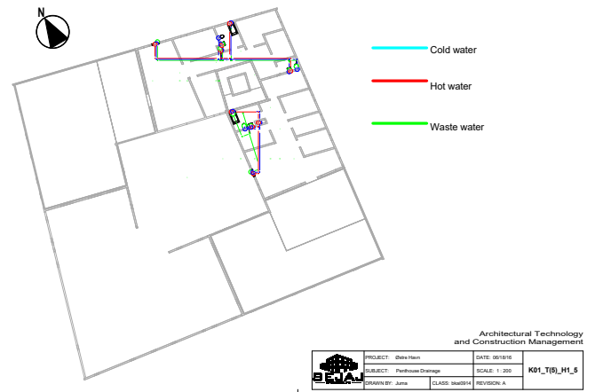
Fig. 131 Water Supply and Drainage Plans: Penthouses Floor
