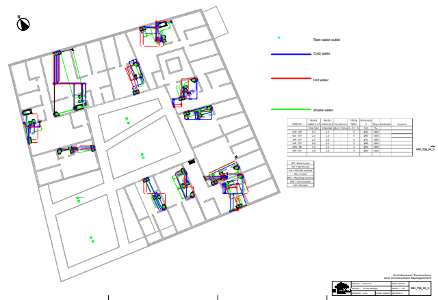
Fig. I29 Water Supply and Drainage Plans: 1 st Floor
