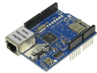
(c) Arduino Ethernet Shield, based on W5100
