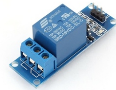
(f) Power Switch, based on SRD-05VDC-SL-C.
