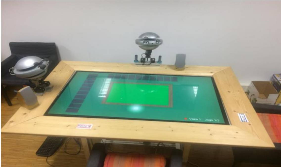
Fig. 1: Multi-touch screen table used to play Sueca and robots in position to play. Speakers were placed next to each robot's head to transmit sound.
