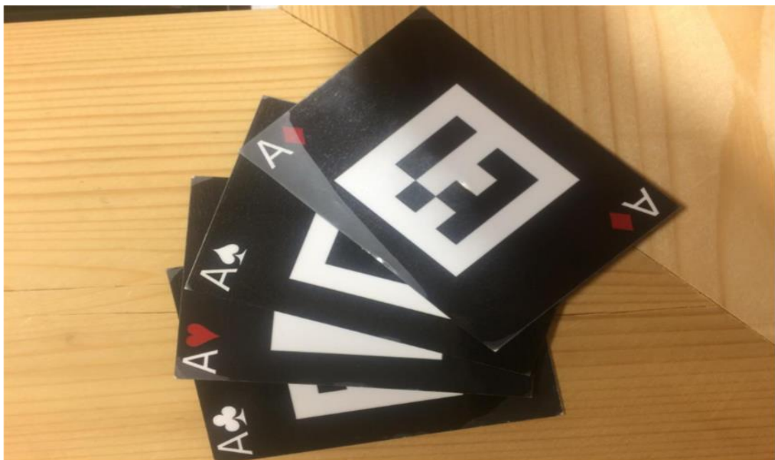
Fig. 2: Cards with fiducial printed markers used to play the game of Sueca.
