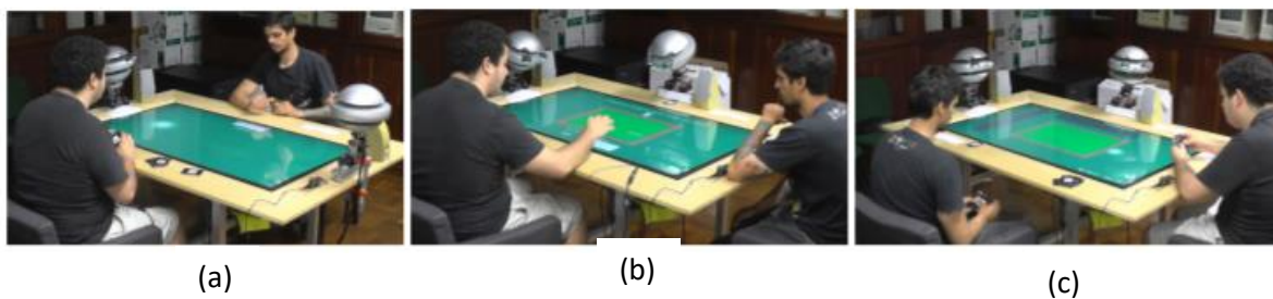
Figure 3: Experimental Setting: Participants play in partnership with one another; (b) Participants play with each of the robots; (c) Participants swap places and play with the other robot. Participants play with a deck of French cards, whereas Robots play with virtual cards and are attached to a multi-touch table and equipped with sound columns, during the course of the game.
