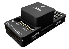
FIGURE 2.7: Pixhawk Cube 2.1 flight controller.
