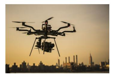
FIGURE 2.5: Multi-Rotor MAV.
