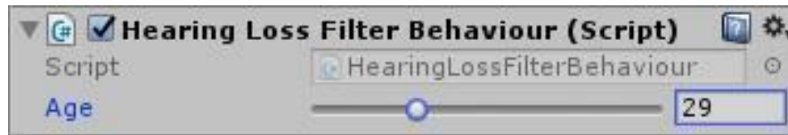
Figure 4.10: The HearingLossFilterBehavior allows the developer to manually input the age of the Listener.
