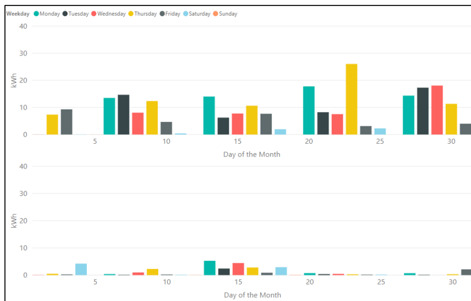
Figure 36 Daily difference in the sum of wasted power between the evaluated auditorium with out-of-reach light switches (upper) and one with user-moderated switches (C103) (lower).
