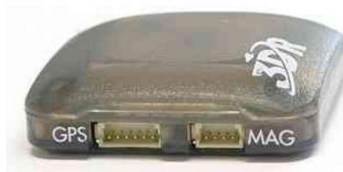
Figure 3-2 - 3DR UBlox GPS + compass module. Source: (Pixhawk Wiring Quick Start, n.d.).
