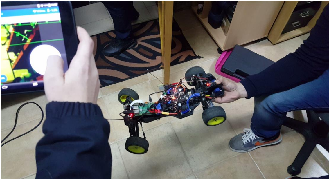
Figure B. 1 – Application being tested with a car, using APMrover2 firmware.
