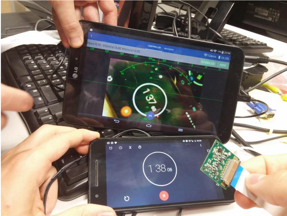
Figure 6-10 - Test case of delay in the video stream.
