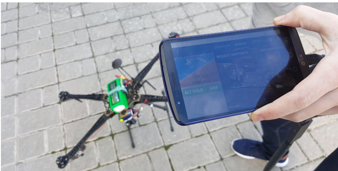
Figure B. 2 – Application tests in a quadcopter, using ArduCopter firmware.
