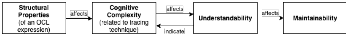
Figure 2.3: Relationship between structural properties of an OCL expression, cognitive complexity related to tracing, understandability and maintainability (based on [14])
