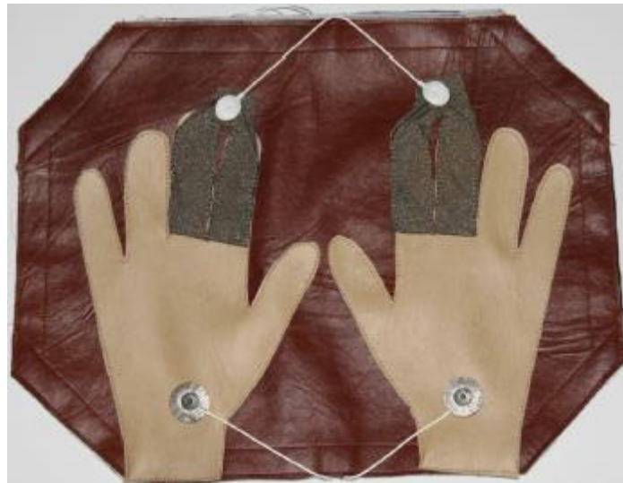
Figure 5 - Electrolycras on the top, dry Ag/AgCl on the bottom (Adapted from Silva et al., 2013).
