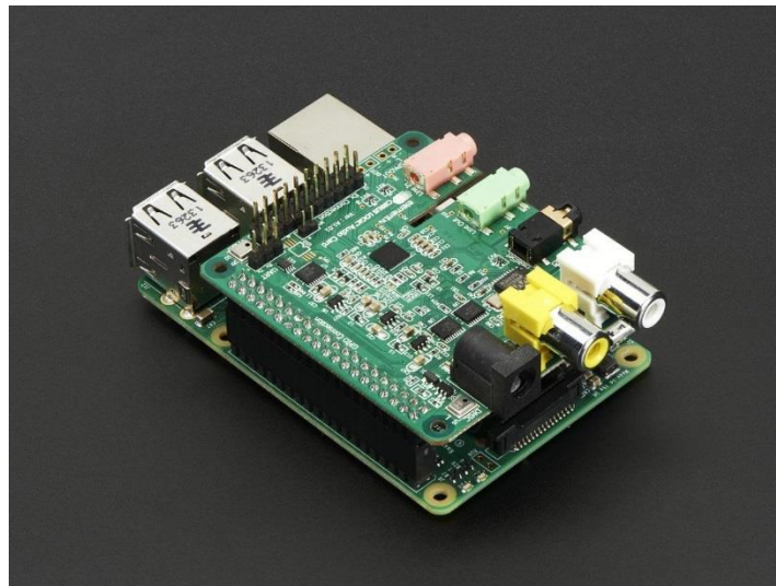
Figure 5 - Cirrus Logic card installation
