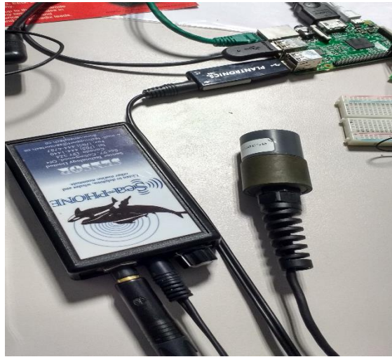
Figure 27 - Hydrophone connected to the USB audio card
