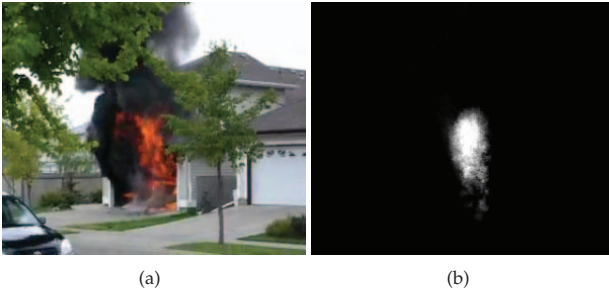
Figure 5. Dynamic texture detection. (a) Input image of a video stream containing fire. (b) Temporal filter output, \mathbf{D}(n) . Brightness is representative of the confidence level stored in \mathbf{D}(n) with respect to the presence of a dynamic texture.
