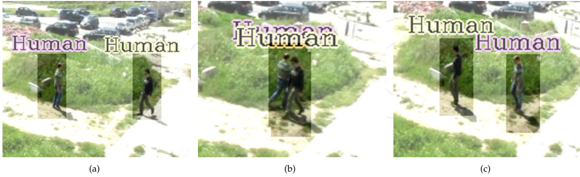
Figure 8. Typical occlusion situation between two moving objects. (a) Moments before occlusion. (b) Occlusion occurs. (c) Moments after occlusion. The objects are successfully associated with the same trackers before and after the occlusion.
