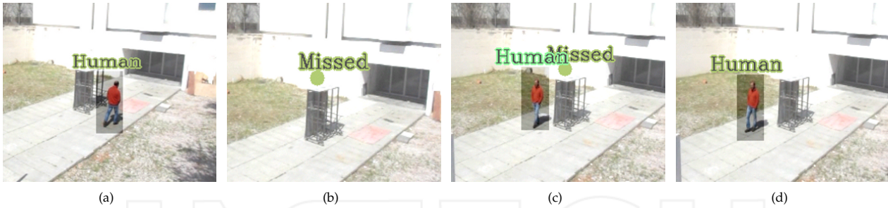
Figure 9. Typical occlusion situation between a moving object and a static structure in the environment. (a) Moments before occlusion. (b) Occlusion occurs. (c-d) Moments after occlusion. The object is successfully associated with the same trackers before and after the occlusion.
