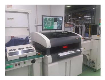
Figure 16 - Production line six AOI
