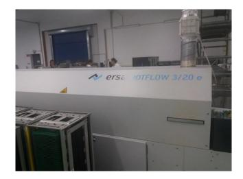
Figure 15 - Production line six Reflow Oven
