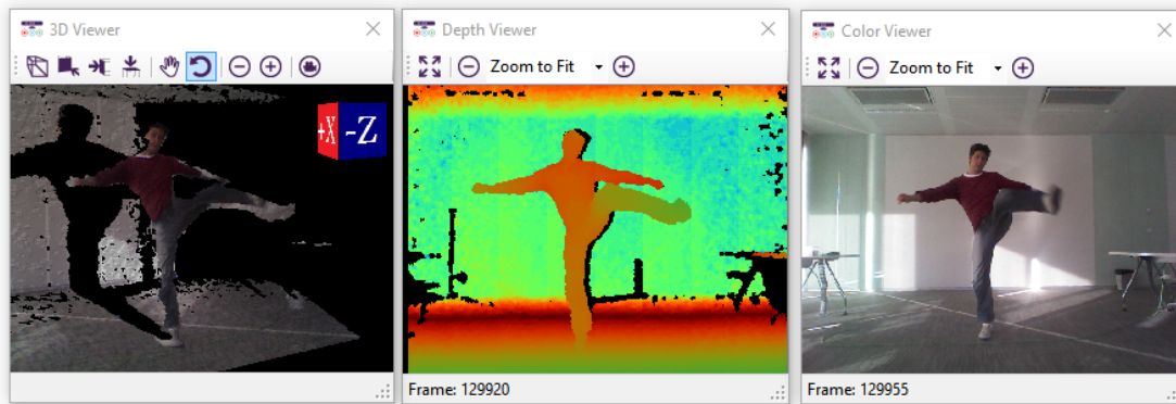
FIGURE 3.10: Microsoft provides visualization tool which allows users to explore the 3D, Depth and RGB view of a recorded .xed file.
