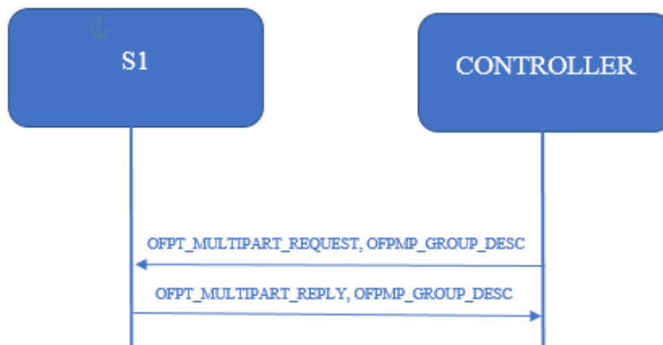
Figure 35: LLDP's Handshake: Step 9
