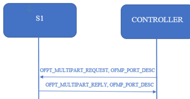
Figure 30: LLDP's Handshake: Step 4
