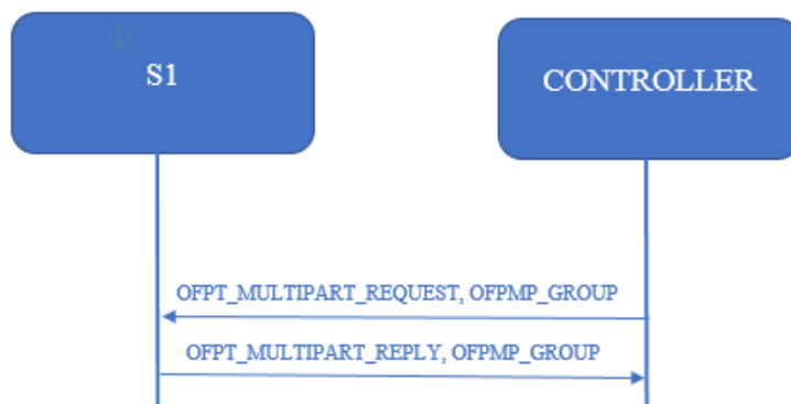
Figure 36: LLDP's Handshake: Step 10
