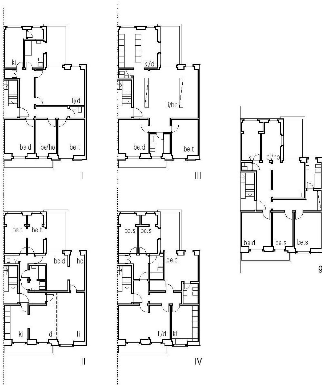
Figure 4: Architect designs (I, II, III, IV) and RB-grammar solution (g) for assignment A.
