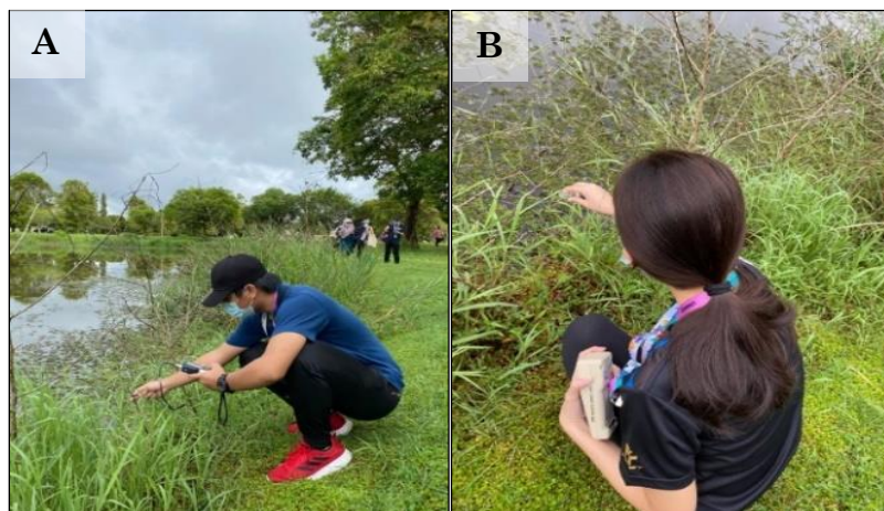
Figure 48. Students measuring the water quality at UNIMAS lake. A. Measuring the conductivity of water using a multi probe. B. Running the turbidity meter to gain the turbidity of water
