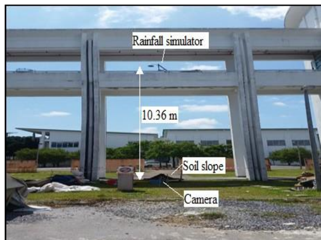
Figure 2 Set-up of rainfall simulator.
