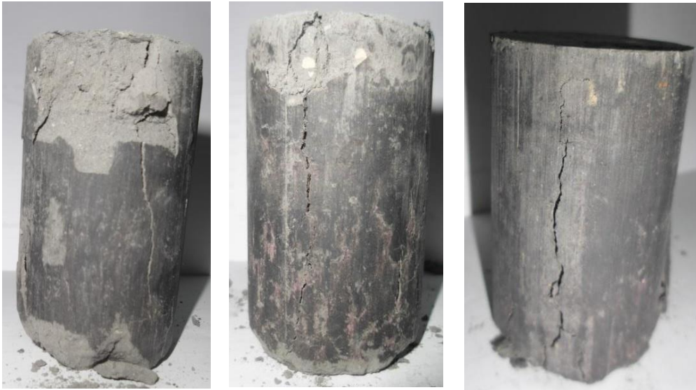
Figure 4: Examples of cracks formation in the mixture of clay-cement
