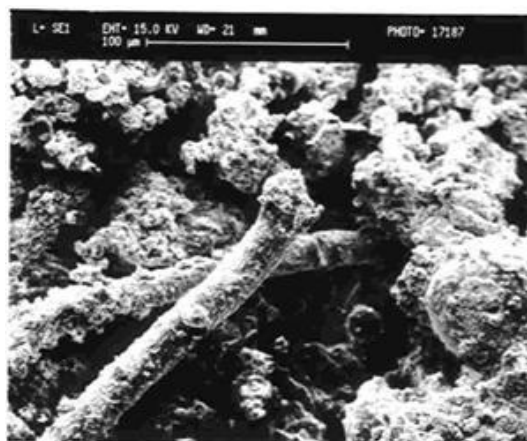
Figure 6 SEM of cement and fiber stabilized Rajghat fly ash – Series II (28 days curing) [24]
