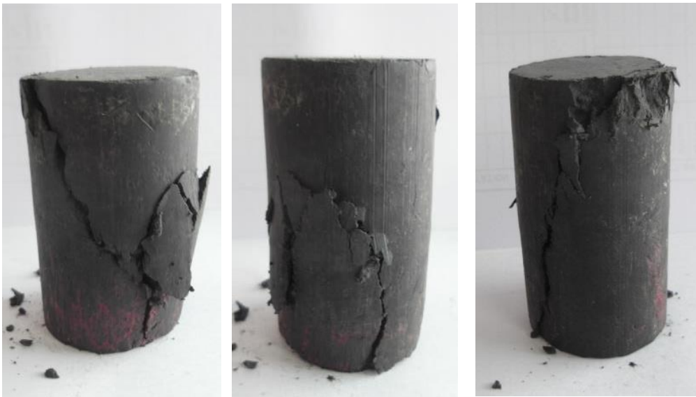
Figure 5: Examples of cracks formation in the mixture of clay-cement-fly ash
