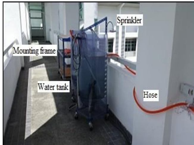
Figure 1 Rainfall simulator and water tanks placed on the 2 nd floor of a building in Universiti Malaysia Sarawak.
