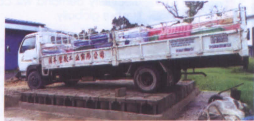
(d) Functionality verification of StormPav green pavement using loaded truck
