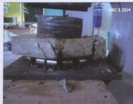
Figure 3: Crushing load capacity determination of cover block using circular load and circular support (Ref. Figure no. 4)
