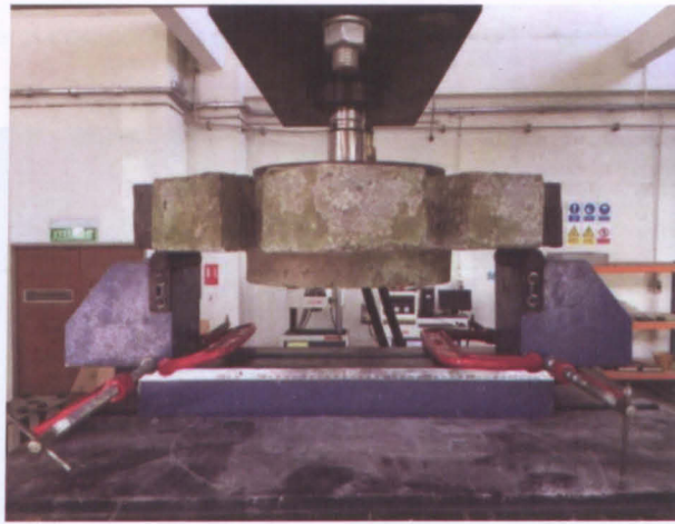
Figure 5: Shear strength determination of Interlocking keys for StormPav blocks
