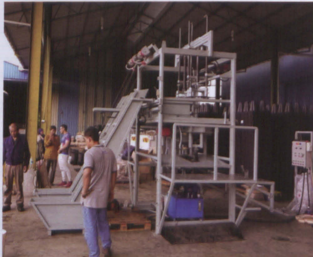
Figure 7: Full-Automated Manufacturing of Hollow cylinder block machine-2
