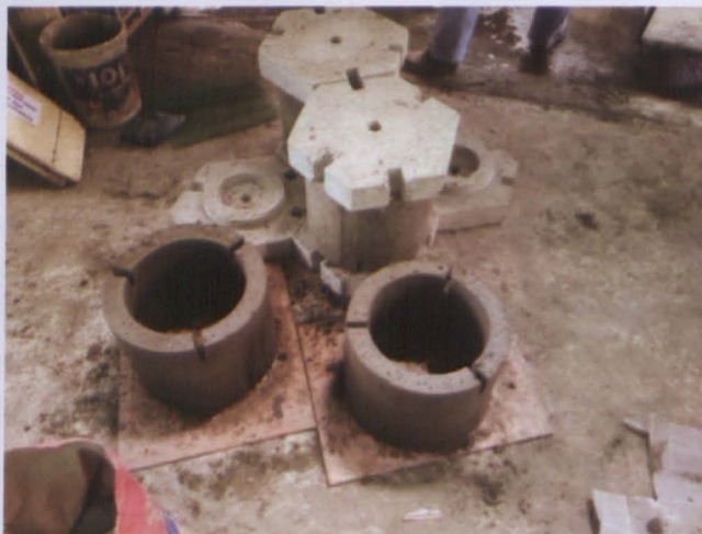
Figure 8: Shape of StormPav blocks made using machines (ref. Figures 6 and 7)
