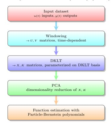
Figure 1. Schematic flowchart of the proposed algorithm.
