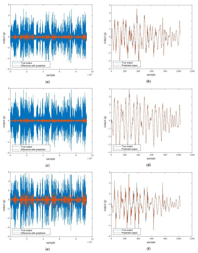
**Figure 4.** (**a**,**c**,**e**) Identification error for testing data of outputs 1, 2 and 3, respectively. (**b**,**d**,**f**) Comparison of true and predicted outputs for a sample window in outputs 1, 2 3, respectively.
