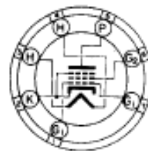
BOTTOM VIEW MINIATURE BUTTON 7 PIN BASE
