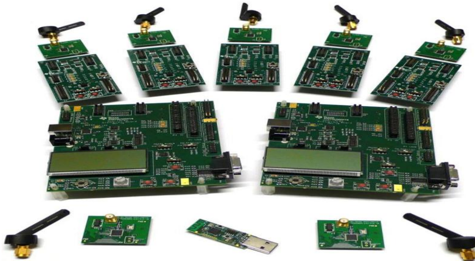
Figura 37. CC2530ZDK ZigBee Development Kit.
