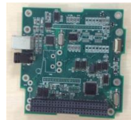
Figure 3. OBC developed at GITEM. Fuente: [16]
