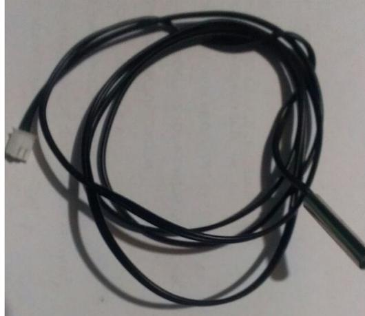
**Figura 11. Termistor NTC  $10K\Omega$**
