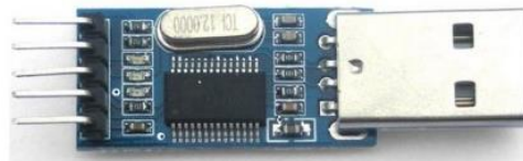
Figura 7. Conversor USB a Serial, TTL UART PL2303. [10]
