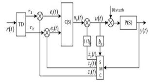
Fig. 3. Show ADRC-based SMC structure
