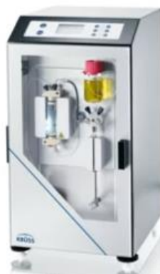
Figure 2.8 Image of a Drop Volume tensiometer. Taken from (122)
