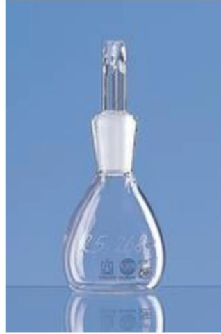
Figure 2.4 Image of a pycnometer. Taken from (117)
