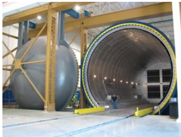
Figure 2.4 - World's largest autoclave, from ASC Process Systems [15]
