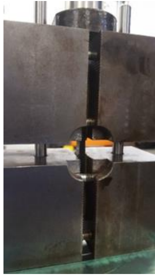
Figure 3.5 - Compression-dedicated fixture used during experimental campaign tests
