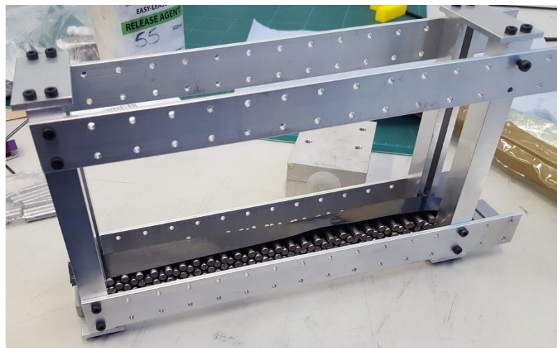
Figure 7.1 - CPCC core manufacturing frame
