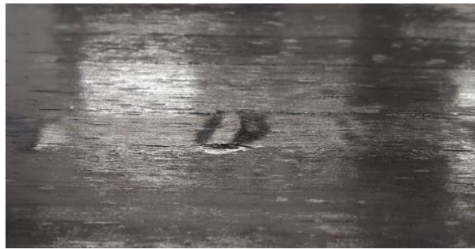
Figure 2.2 - Air package entrapped between prepreg layers during hand lay-up
