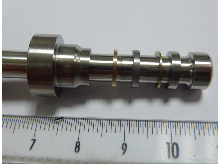
Figure 4. View of the modified Bridgman unsupported area seal used for the Ti-Zr high-pressure cell during its assembly. Mounted on the mushroom plug are (from right to left) the front-packing ring, first anti-extrusion ring, soft central ring, second anti-extrusion ring, and back-packing ring. The numbered ruler markings are on the cm scale.
