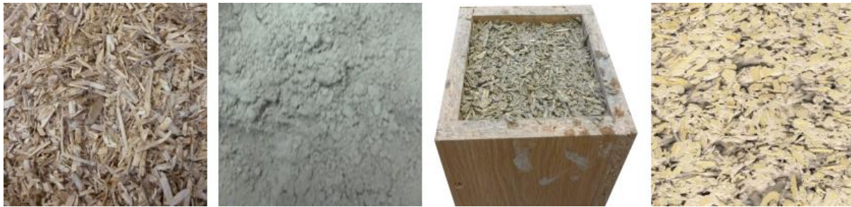
Figure 1: Stages of hemp-lime production: Hemp shiv, powdered lime binder, cast wet material, resultant dried material
