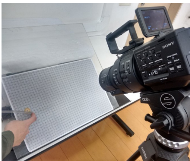
Figure 1. Perspective photography of the experimental arrangement. The camera was aligned perpendicularly to the inclined plane and the coin launching was done with the aid of an acrylic ruler.
