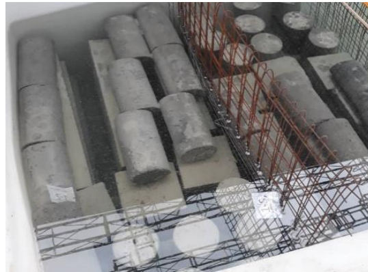
Fig. 2. The curing of concrete samples in water.
