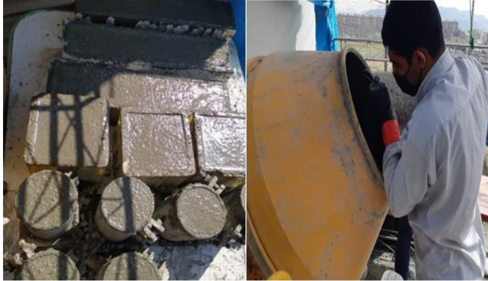
Fig. 1. The concrete preparation samples in the laboratory.
