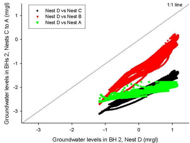
Fig. 7. Correlation between BH 2 (~10 m) groundwater levels at Nest D and Nests C to A.
